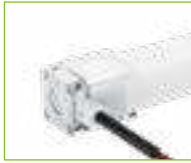
DIY End Cap 2PIN Order Code: 1617S-WS-C-2P-S/L-30 Dimension: 30x20.8x21.4mm/ 1.18"x0.82"x0.84"(LxWxH) Color: transparent Cable Entry: Left side
