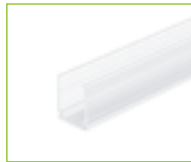
PC Profile Order Code: AC167-PC Dimension: 1000x19.5x22.6mm/ 39.37"x0.77"x0.89"(LxWxH) Material: polycarbonate Color: transparent
