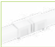
Strip to Strip Connector IP54 Order Code: 1617T-NS-J-4P Dimension: 55x20.8x21.4mm/ 2.17x0.82"x0.84"(WxH) Material: polycarbonate
