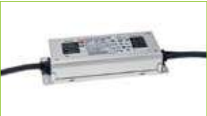
Order code: XLG-150-24-A AC100-305V DC24V 150W IP67, Global certification. Non Dimmable.
