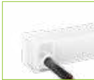
End Cap 2PIN Order Code: AC167A-EC2-S Dimension: 14x19x19mm/ 0.55"x0.75"x0.75"(LxWxH) Color: transparent Cable Entry: side
