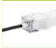
DIY End Cap 4PIN Order Code: 1617S-WS-C-4P-F/L-30 Dimension: 30x20.8x21.4mm/ 1.18"x0.82"x0.84"(LxWxH) Color: transparent Cable Entry: Left front
