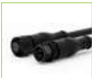
IP67 Connector 2PIN Order Code: AD007-2 Wire Gauge: 0.519mm 2 /20AWG Protection: IP67 (Mated) Mechanical Operation: >500 mating cycles
