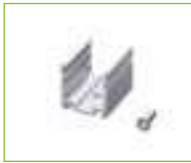
Mounting Clips Order Code: AC167-MC Dimension: 25x20.2x20.8mm/ 0.98"x0.80"x0.82"(LxWxH) Material: aluminium Color: silver Each meter led strip needs 4 clips + 4 screws
