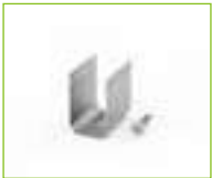
Mounting Clips Order Code: AC016-SET Dimension: 20x13x19.2mm/ 0.79"x0.51"x0.76"(LxWxH) Material: stainless steel Color: silver Each meter led strips needs 4 clips + 4 screws
